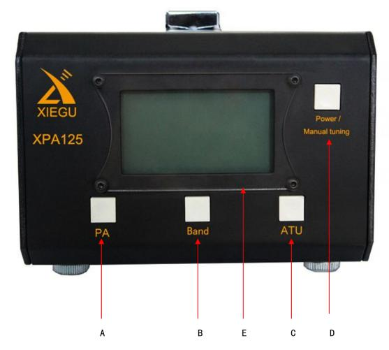
A. PA function key, in the "BYPS" state, press the key, enter the "INUSE" state; in the "INUSE" state, press the key to enter the "BYPS" state
